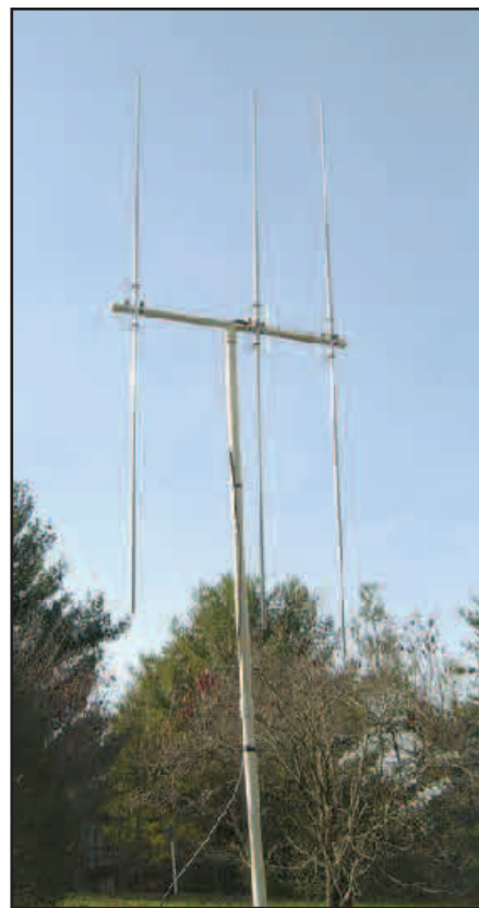
Figure 1 — The prototype 3 element wideband phase-fed Yagi on the test mast. Note that this mast is nonconductive to avoid interactions with the nearby driver elements.
